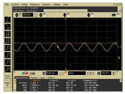
Figure 1. Waveform of a ring oscillator through the switching matrix of the Agilent 4080 test system
